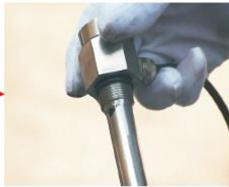
8. Installing O-Ring on the sensor
