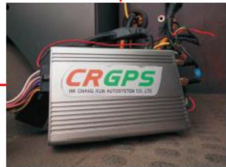
10. Installing the smart terminal Equipment
