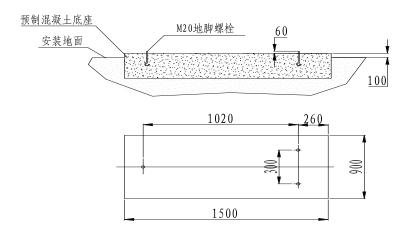
The above dimensions are all counted as per unit(mm). Concrete height as per floor condition, generally no less than 500mm.
