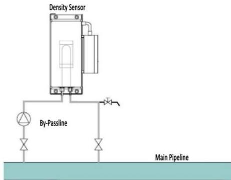
Based on actual case, Tosilon will provide the installation drawing accordingly. This chart is for reference
