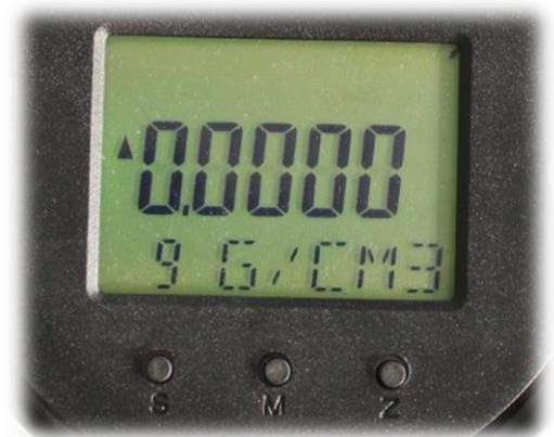
Press and hold "M" for 5 seconds, the display will turn to "Setting Interface". As picture shown
